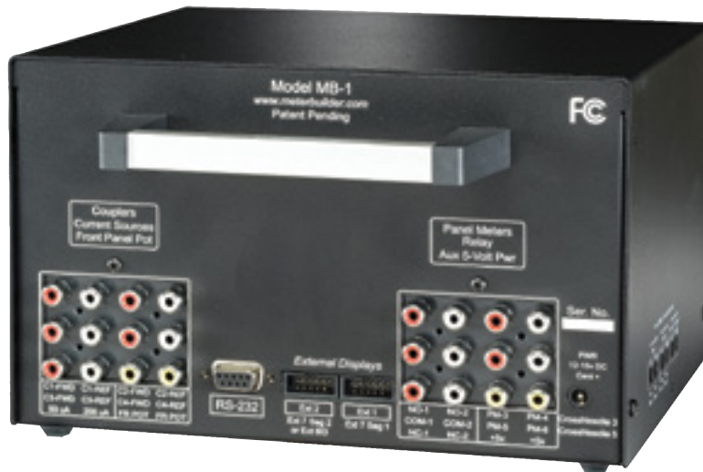
Figure 5 — Looking at the back of the MB-1, you can see lots of phono jacks for coupler inputs and external meter outputs as well as a number of test signals and auxiliary power. The pair of ICD connectors is for the external 7-segment display and bar graph. There is also an RS-232 serial port that you can connect to a computer for firmware updates.
